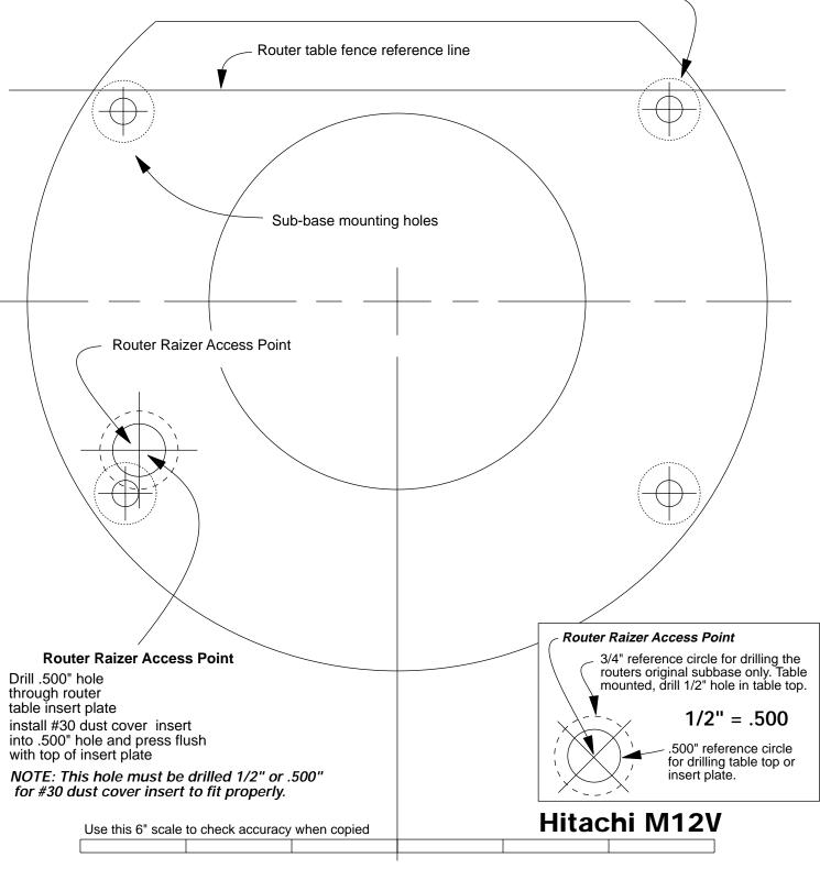
*Note:* Cross lines for locating and drilling holes are accurate. The illustration of subbase may vary slightly in size and design, but is accurate enough for cutting the rubber gasket if required.
