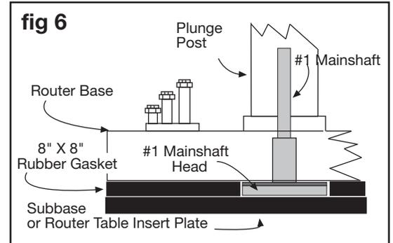
**Installing the Dust Cover Insert**
